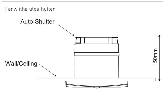
When fitted, the duct outlet must be the same height or higher than the exhaust fan.
